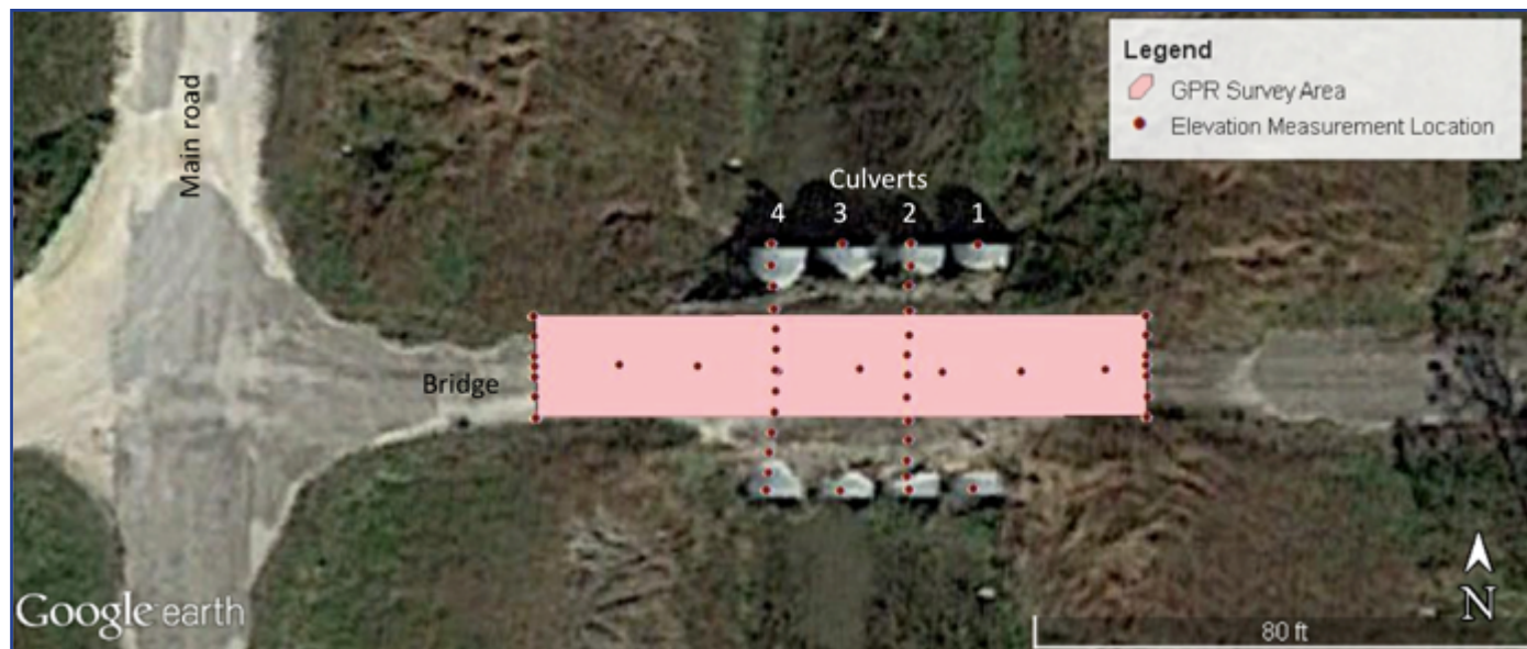
Figure 1: Map of survey area showing elevation data positions (dots) and GPR survey grid area (pink rectangle), UH Coastal Center La Marque, TX. (Map Source: Google Earth.)
